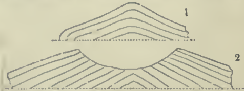
1. Anticlinal line forming the crest of a hill. 2. The same line running along the course of a valley.
